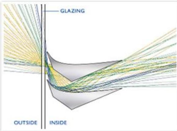
The patented LightLouver reflective slat design redirects all sunlight above a 5 degree altitude angle upward onto the ceiling of the daylit space, providing ambient lighting and eliminating direct sunlight on work surfaces. LightLouver units are a perfect solution for East, West and South facing windows.
